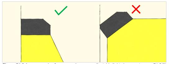
Figure 71.2.1: an example of proper vs. improper adjustable light placement as per 71.2(3) of this section.
