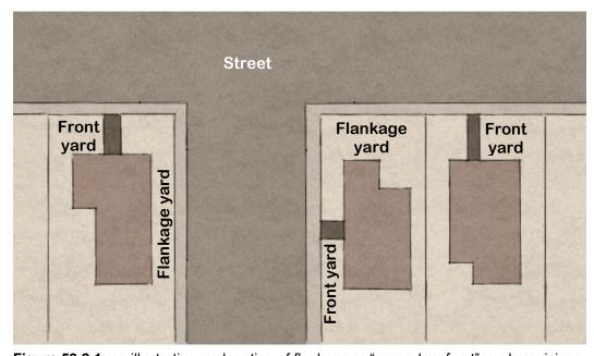
Figure 59.2.1: an illustrative explanation of flankage or "secondary front" yard provisions.
