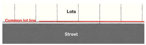
Figure 60.3.2: an example of a common lot line as per 60.3.1(e) of this section.
